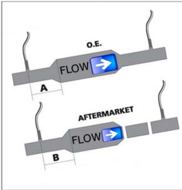
In order to ensure converter light-off, the front of the replacement converter should be installed as close to the OEM position as possible.
